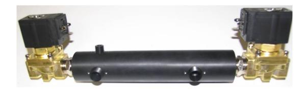
The biological material is introduced into a Delrin tube by a solenoid injection valve; optical sensors allow to measure the fluorescence emitted by chlorophyll inside the green algae cells in culture medium and the density of the these cells culture medium through a light transmission measurement. It is equipped with current measurement system, and an electronic control board for data read-out, processing and PC transfer.
